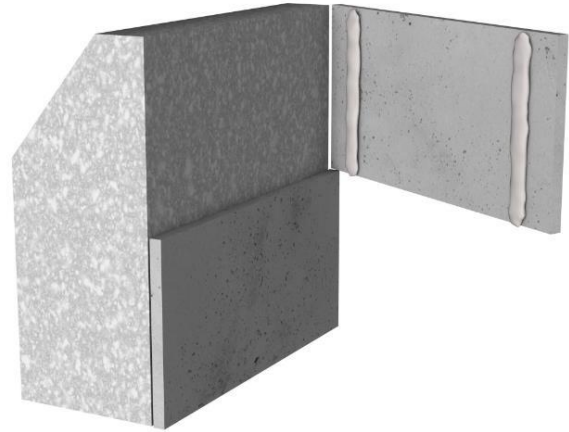
Example of gluing with dispersion glue
